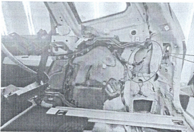
Inner view of panel indicating pieces of wire welded to the fender and body filler used. Causing deformation of right rear fender.
